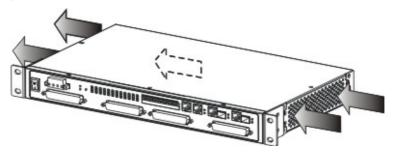
Figure 3-1 NCT480 Ventilation Control Diagram
